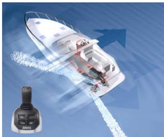
With the joystick the driver can maneuver the boat, at low speed. The joystick is coupled to a sophisticated and specially developed software that individually commands the electronically controlled engines and underwater units of the system to steer, throttle and shift gears independently, making the boat move in any direction the driver wants – sideways, diagonally, forward, backward or rotate – with just one hand. Visit [volvopenta.com](http://volvopenta.com) to see for yourself!
