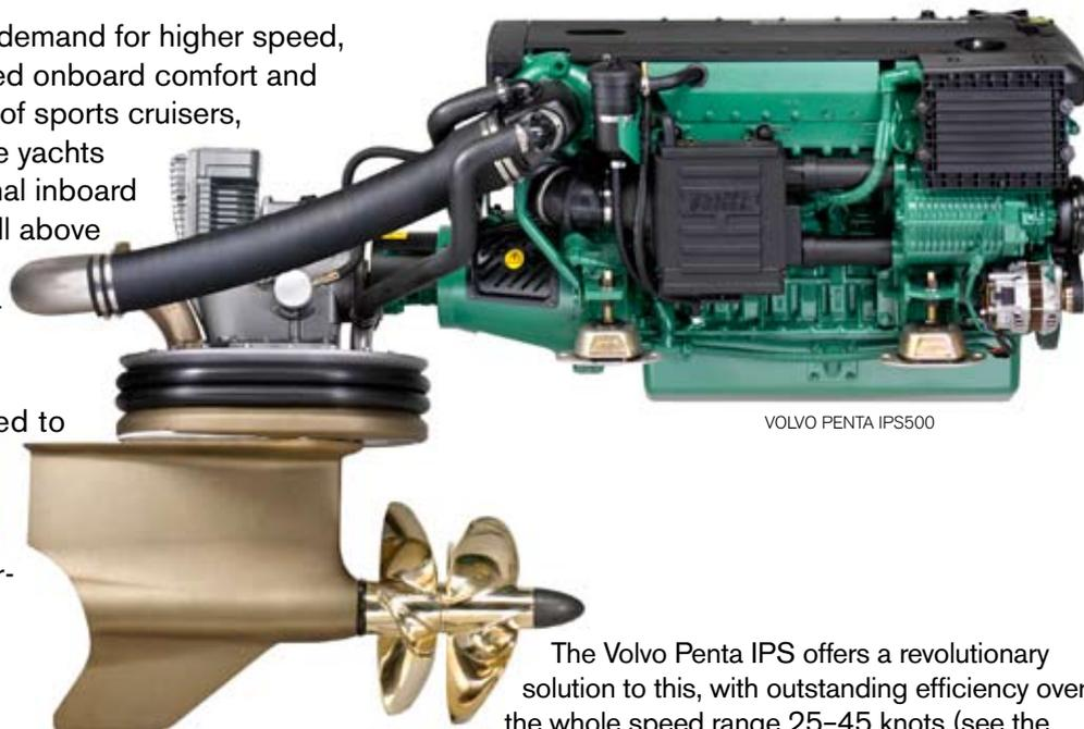
The Volvo Penta IPS offers a revolutionary solution to this, with outstanding efficiency over the whole speed range 25–45 knots (see the upper curve in below diagram).
